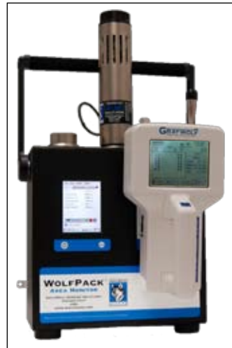
▲ WolfPack shown with PC-GW6 6-channel Particle Counter (GrayWolf PC-3016)
